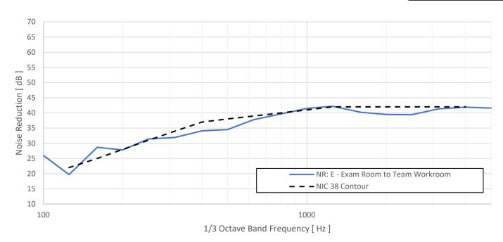
Figure C.5: Noise reduction of partition between Weill 253B and Weill 253C
