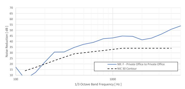
Figure C.6: Noise reduction of partition between Weill 581H and Weill 581G
