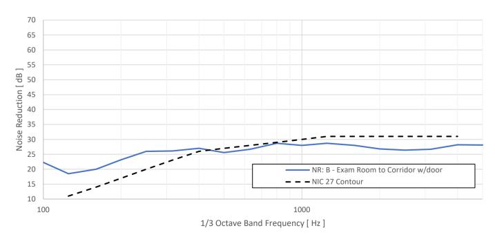
Figure C.2: Noise reduction of partition between Weill 252B and Weill Corridor
