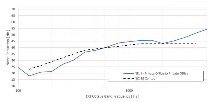
Figure C.10: Noise reduction of partition between Weill 511F and Weill 511E
