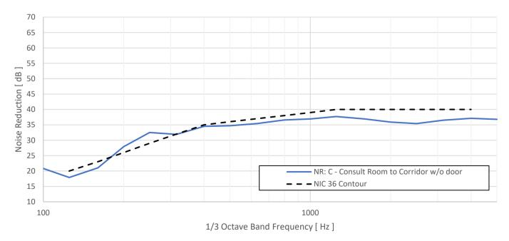
Figure C.3: Noise reduction of partition between Weill 254A and Weill Corridor
