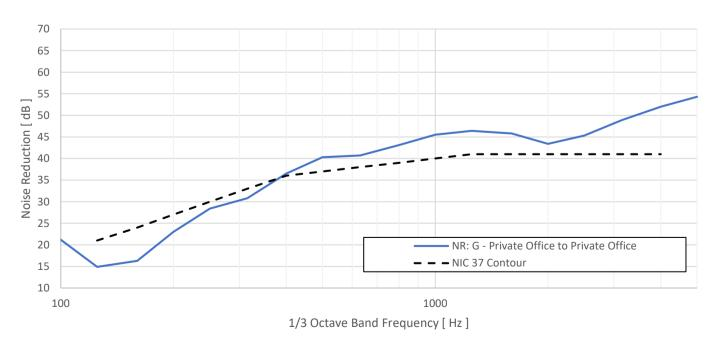
Figure C.7: Noise reduction of partition between Weill 581H and Weill 581J
