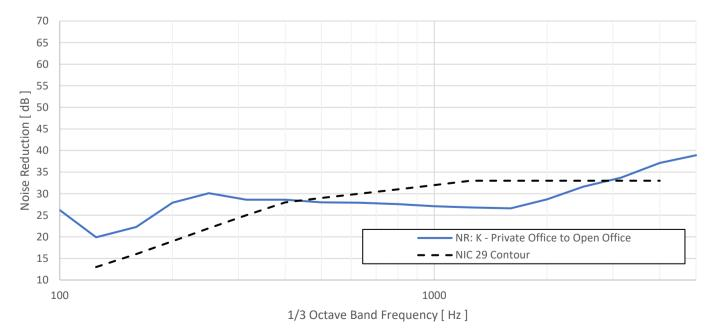
Figure C.11: Noise reduction of partition between Weill 511F and Weill 51306
