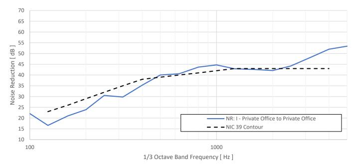
Figure C.9: Noise reduction of partition between Weill 511F and Weill 511G
