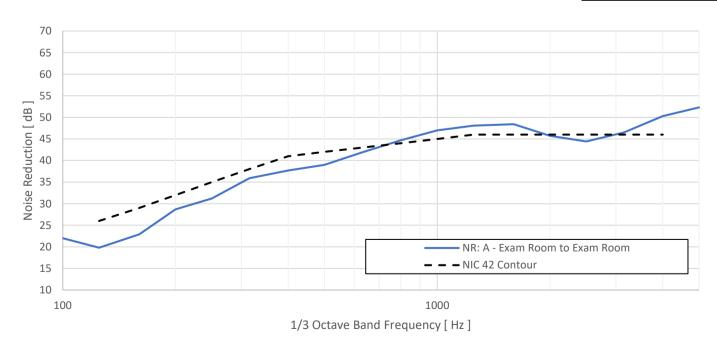
Figure C.1: Noise reduction of partition between Weill 252B and Weill 252C
