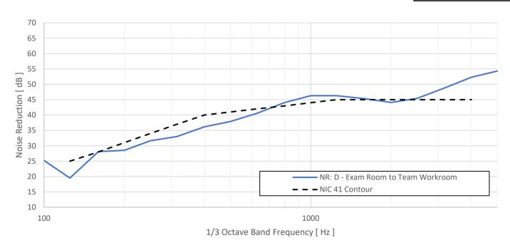
Figure C.4: Noise reduction of partition between Weill 253B and Weill 253C
