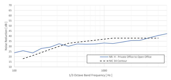
Figure C.8: Noise reduction of partition between Weill 581H and Weill 58505
